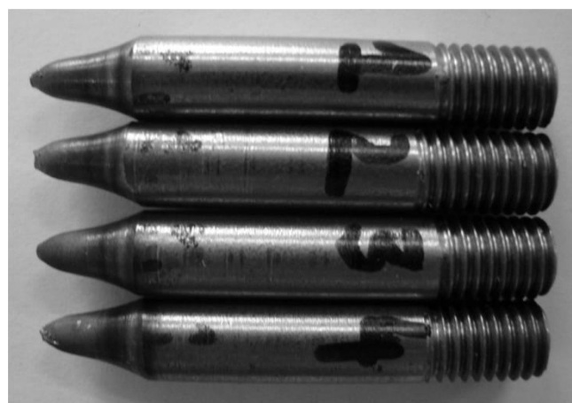
Fig. 8. View of C45 steel samples broken in a tensile test using the Gleeble 3800 simulator at 1 - 900°C, 2 - 1000°C, 3 - 1100°C, 4 - 1200°C
