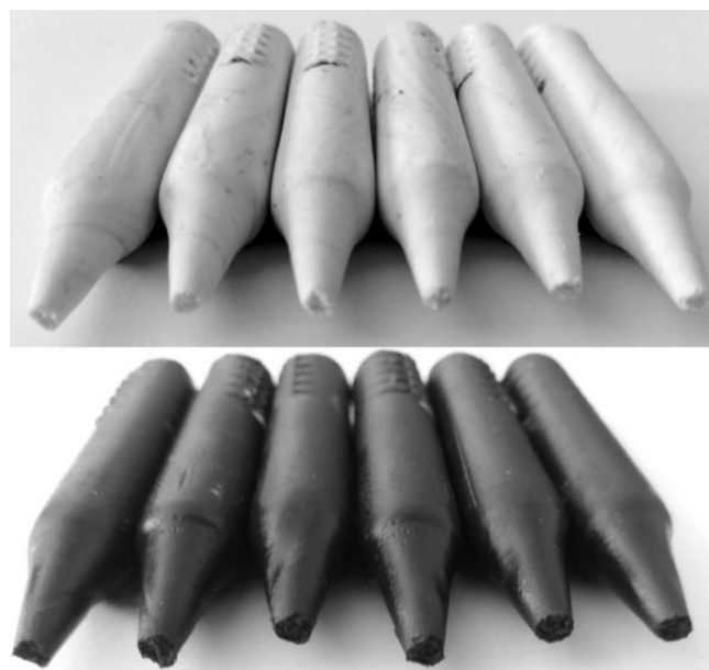
Fig. 7. View of plasticine samples broken on a testing machine
