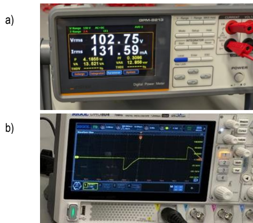
Fig. 8. Real object test results: a) power and power factor measurement, b) signal waveform on a resistive load
