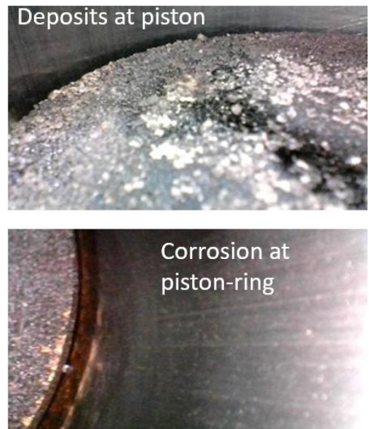
Fig. 11b. Endoscopy of combustion chamber [26]
