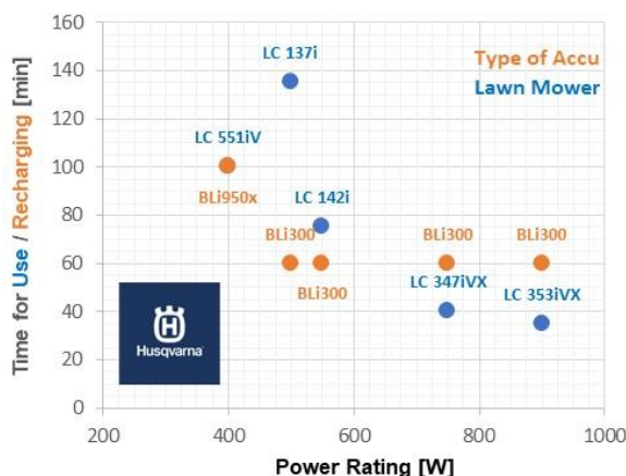
Fig. 1b. Time for use/recharging of lawn mowers
