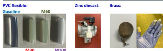
Fig. 13. Results of material tests [26]
