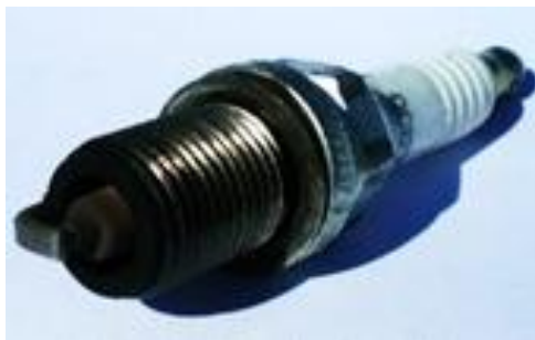
Fig. 11a. Sparkplug after methanol operation
