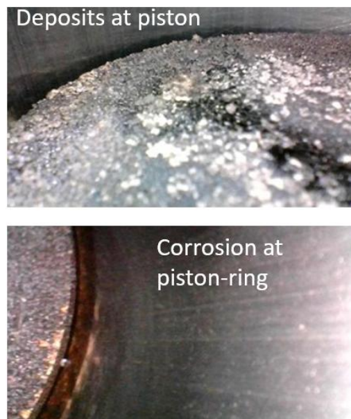
Fig. 11b. Endoscopy of combustion chamber [26]
