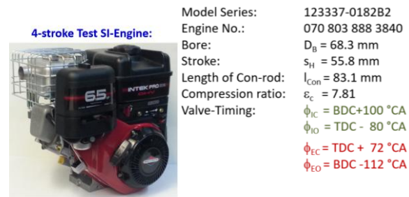
Fig. 4a. Test-engine Briggs & Stratton Intek Pro 206
