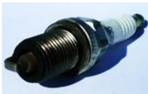
Fig. 11a. Sparkplug after methanol operation
