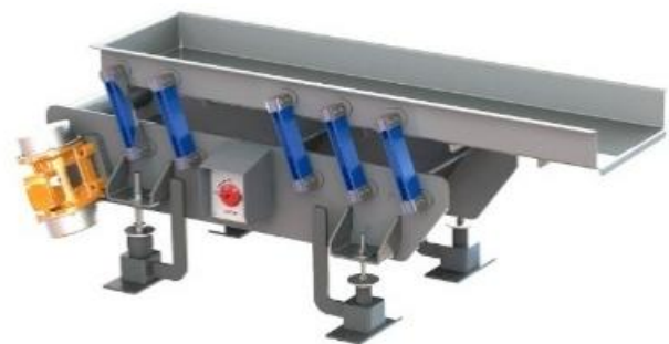
Fig. 1. VIBRAflex II Sanitary Antiresonant Vibratory Conveyor – PFI, which dynamic and discrete model is presented in Fig. 2
