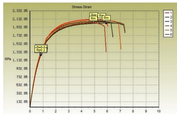
Fig. 29. The results of the tensile tests
