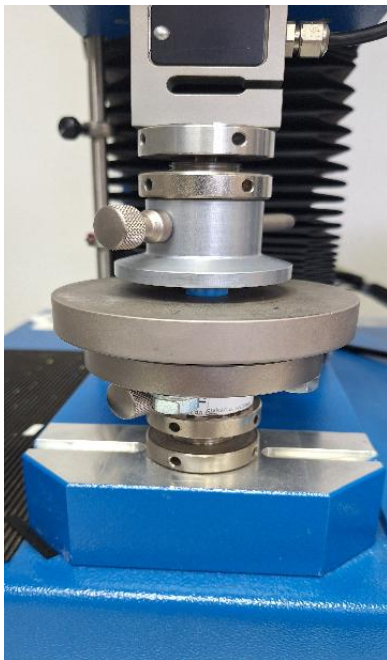
Fig. 4. View of the stress relaxation test
