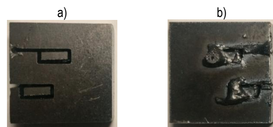
Fig. 1. An attempt to cut out samples from S355J2C+N steel using the manufacturer's parameters: a) surface view, b) underside view
