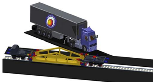
Fig. 4. Stage I of loading – entry of the wagon onto the railway platform adapted for loading semi-trailers, positioning the tractor in the loading area and preparing the wagon for the rotation of the loading platform
