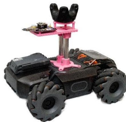
Fig. 8. Robomaster S1 robot with tracker mounted
