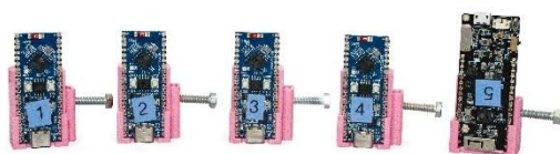
Fig. 7. ESP32 units used as APs
