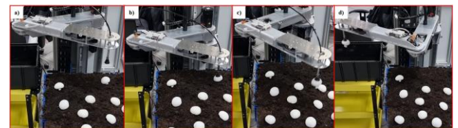
Fig. 19. Typical operating cycle: a) finding a mushroom; b) picking, c) and d) moving to bin
