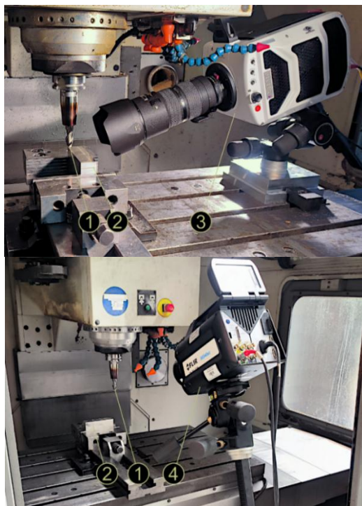
Fig. 2. Research setup (1 – end mill, 2 – workpiece, 3 – high-speed camera, 4 – thermal imaging camera)
