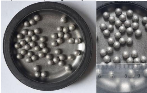
Fig. 9. Milling balls after mechanical alloying of the Ni–20 wt% Cr mixture in the Pulverisette 6 mill for 15 h
