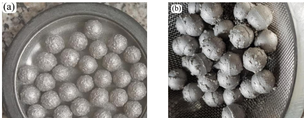
Fig. 5. Milling balls after mechanical alloying of (a) Ni–20 wt% Cr and (b) Ni–20 wt% Mo mixtures in the AIR planetary mill
