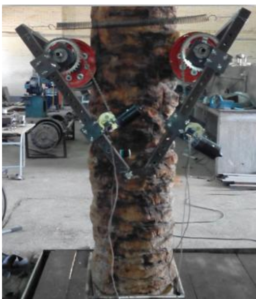
Fig. 5. Climbing device with hinged V-shaped chassis for ascending date palm trees
