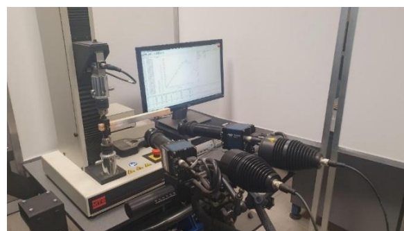
Fig. 4. MTS Insight measurement station with a DCB sample attached, together with the ARAMIS 3D 4M measurement system
