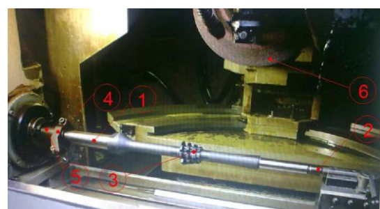
Fig. 6. Grinding process of the tool – hobbing cutter on the machine (1 – tool – hobbing cutter; 2 – clamping tips; 3 – tool groove; 4 – drift pads; 5 – headstock; 6 – grinding wheel)
