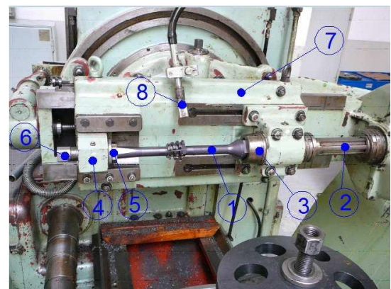
Fig. 4. Clamping the workpiece in a special fixture (1 – tool – hobbing cutter; 2 – tool headstock; 3 – drifting part; 4 – backing bearing; 5 – plain bearing; 6 – nut; 7 – tangential support; 8 – cooling tube)
