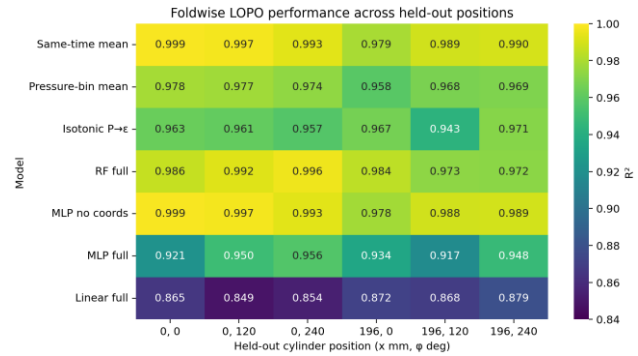
Fig. 6. Position-wise R^2 values for representative methods across the six held-out cylinder locations. The figure describes sensitivity to the selected sensor position within the same burst event; it is not a cross-vessel validation map
