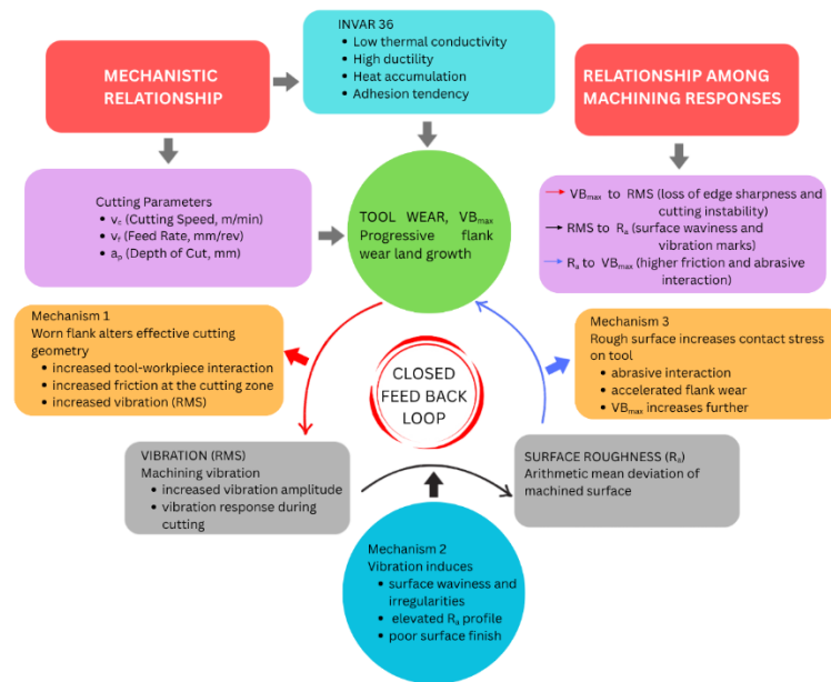
Fig. 10. Mechanistic feedback-loop illustrating the interrelationship among tool wear ( VB_{max} ), machining vibration (RMS), and surface roughness ( R_a ) during dry turning of Invar 36
