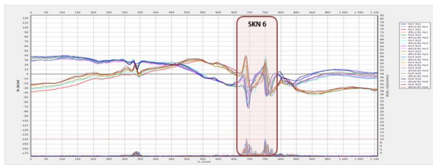
Fig. 11. Distribution of the tangential H_{xi} and normal H_{yi} components of the magnetic field strength [A/m] and their gradients dH_{xi}/dx , dH_{yi}/dx , i=1-6 [A/m/mm] along the measurement length [mm]: a) SCZS 5 magnetogram; b) SCZS 6 magnetogram
